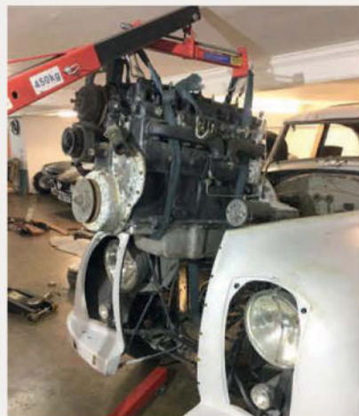
The engine was removed and rebuilt, and is now running as it should – for the first time in a long time.
