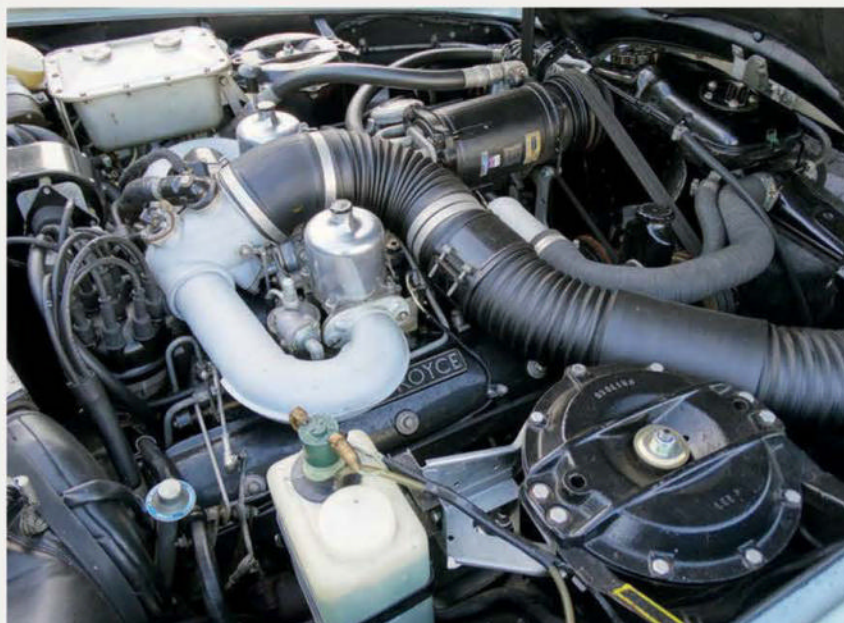
The Silver Shadow inherited its predecessor's 6.2-litre L-series V8, later increased to 6.75-litre capacity.
