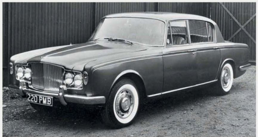
The front-end treatment of this Bentley Burma concept featured a full-width grille design incorporating quad headlamps.
